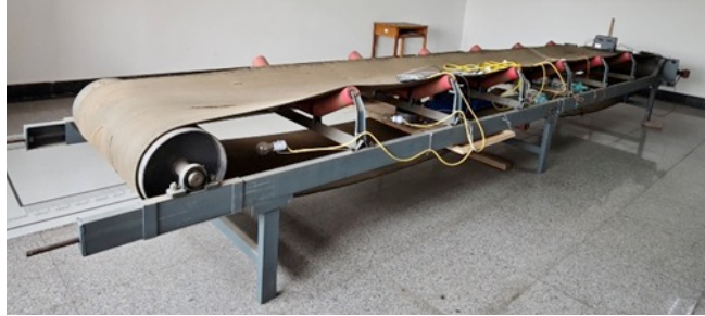
Figure 3: Simulation apparatus for conveyor belt tear failures
